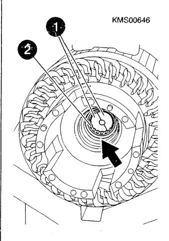
Replacing needle bearing in armature Removing (continued):
